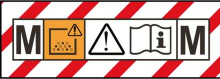
The device is suitable for vacuuming dusts up to dust class M.
