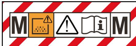
The device is suitable for vacuuming dusts up to dust class M.
